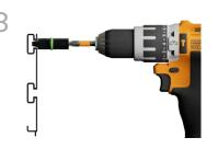
Place screw guide into channel at stud location. Firmly press both guide and drill against rail and drive screw through channel into stud. 9 10
