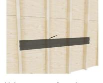
Using your preferred method, locate and mark every stud along the line. NOTE: Studs must be within 7" of the end of the rail. When joining rails end to end if a stud aligns with joint of the two rails, move display 1" left or right.
