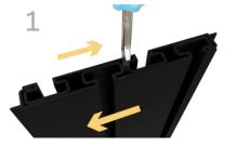
Rails will be nested back-to-back for safe shipping. Be sure to separate before assembling. (It may be necessary to use a screwdriver to separate rails) 2
