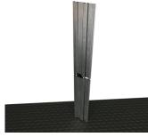
Insert connector plate into back of slatwall. Press rails together. Grasping the top rail, tap rails on a rug or a non-maring surface to close gap.
