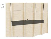
Extend lines vertically to the full height of the 36" display and recheck stud alignment.
