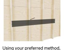
locate and mark every stud along the line. NOTE: Studs must be within 7" of the end
