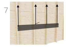
Mark lines vertically to the full height of the display and recheck stud alignment.
