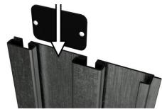
Insert connector plate into back of slatwall.
