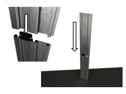
Press rails together. Grasping the top rail, tap rails on a rug or a non-marring surface to close gap.
